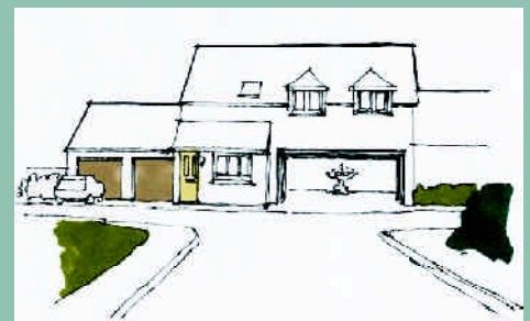
Access to backland development can be via an archway under frontage development. The view through the archway should focus on an attractive feature and not parked vehicles
